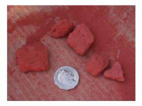
Not all phosbins have this problem. Investigation is underway to gather details on occurrences, and serial numbers to isolate production runs that have been contaminated. A system of sieving phosbins to strain out any phosrocks has been set up and re-sieving of old stock is underway.
